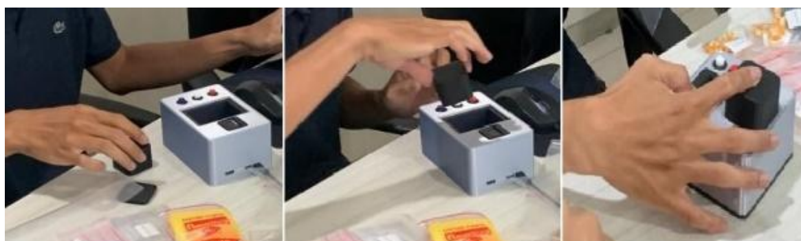
Figure 4. Spectral data measurement procedure for maize seeds using Vis/NIR
